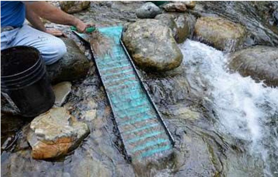
High banker – A form of sluice box, usually in two parts comprising of a header box and sluice box below. Water is pumped to it and gold bearing material is fed into the header box which screens out the oversize rocks and pebbles and allows the water and fines to run through the sluice box. Here is a picture.
