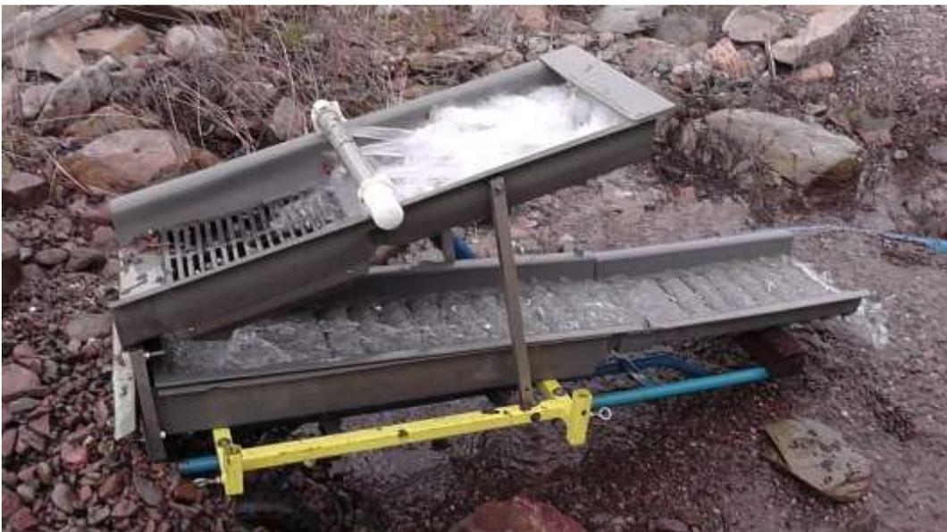
Dry-blower – traditionally used in desert areas and uses air and agitation to settle gold-bearing concentrates. Can be adapted for use with small portable motorised air pumps in the same way that motors are used in high-banker sluices.
